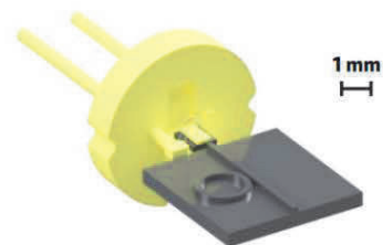
Self-injection locking of Fabry-Perot LD (Seminox, < 300 mW) to the high-Q microresonator (Ligentech, Q > 10^6 )
